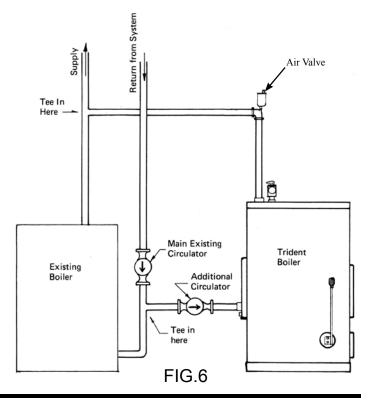
The circulator installed between the two boilers may be hooked up to run continuously during the heating season or, an additional S350 control (not supplied) could be installed to turn it on and off automatically. This control must be used as a "close on rise of temperature" (jumper in cooling position).
